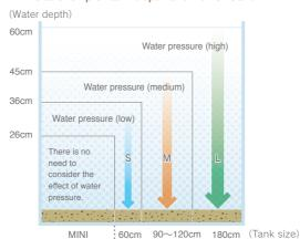
Chose Power Sand based on the height (water depth), instead of the size of an aquarium. S
